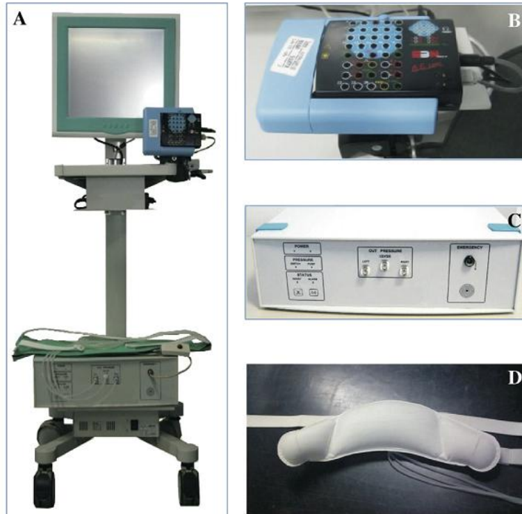
Fig. 2. Baby-guard composition. (A) The Baby-guard device with (B) the equipment for fetal heart-rate monitoring, (C) the pump for the belt, and (D) the belt.
