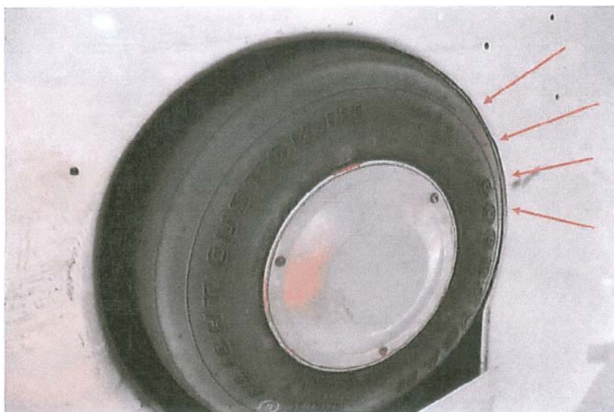
Picture 3: interference signs on the airframe close to the left main landing gear.
