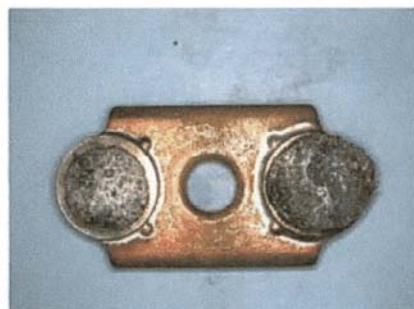
Picture 5 : relay R2-63 A1 contacts.
