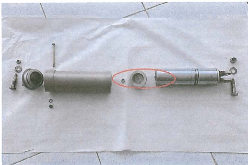
Picture 2: left main landing gear shock absorber disassembled.
