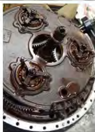
Foto 4: quill shaft e reduction gearbox .
